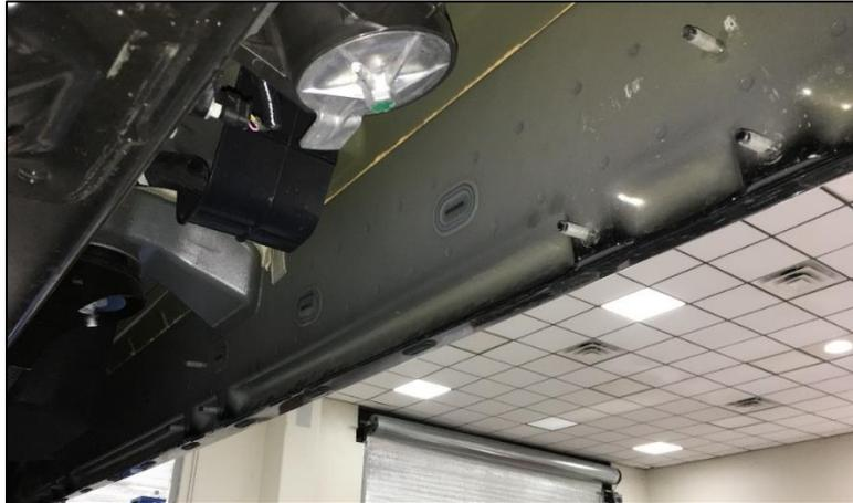
**Step 4:** On the inside rocker panel there will be three-attachment point consisting of three 8mm studs coming out from the panel. These studs may be covered in paint and will need to be cleaned before the installation.
