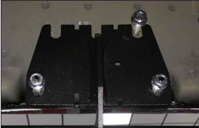
**Step 6:** Next, adjust the Hoop step level with the body of the cab and tighten all hardware 30 ft. /lbs.
